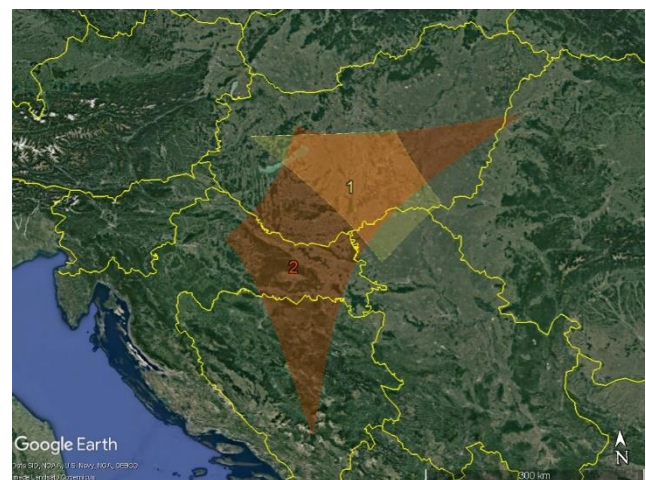
Figure 16 – GMN camera fields in 2022 intersected at 100 km elevation, for cameras active in Hungary. The code refers to the camera ID, e.g., 2 = HU0002.
