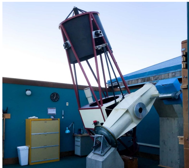
Figure 3 – FPOA “Challenger” 1-meter f/3.58 telescope has been in operation since 1986.
