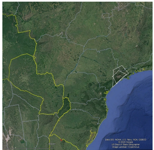
Figure 11 – Global Meteor Network camera fields intersected at 100km elevation, for cameras installed in Brazil.
