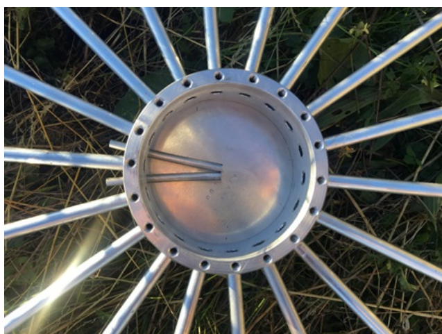
Figure 3– BOS, Observing station Bos-cha, the center part with two output tubes: One for the Infiltec Infra20 sensor and another one for the Raspberry Boom sensor.
