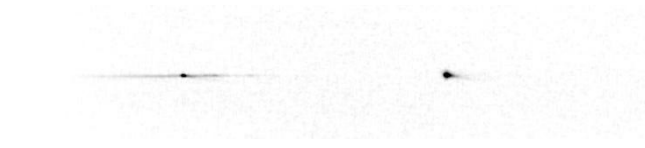
Figure 10 – Spectrum recorded at Gnosca. Meteor moving to the left, first order at other side of zero order compared to MAI_2, therefore the meteor train pointing in the other direction with respect to the spectrum. 50 fields added.
