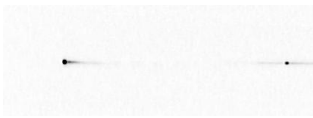
Figure 9 – M20170102_015202_MAI_2.jpg, 170 fields added after background subtraction, linearization and registration.
